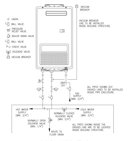
**Drain Solenoid Piping (Fig. 3)**
